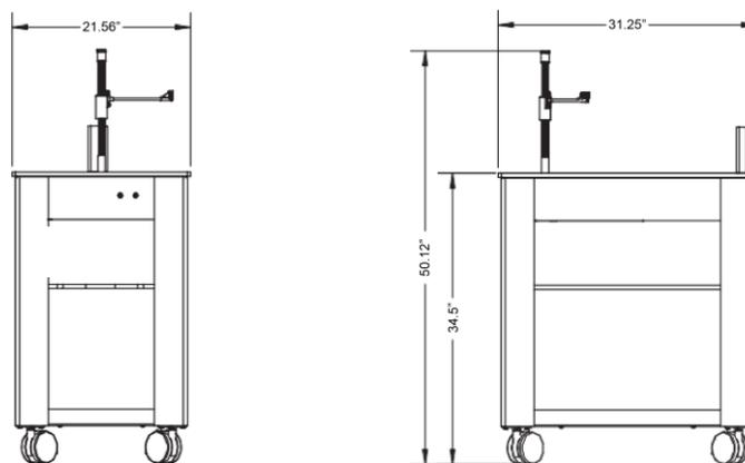
SC-8DX Autosampler with ULPA Filtered Enclosure
